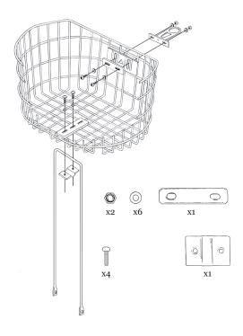
Assemble the basket as illustrated. Thread the lower stays on the wheel axle (outside washers) and put the wheel nuts in place. Before proceeding to the next step now check that the parts are assembled in the correct order: wheel-front fork - washer - stay - wheel nut.
