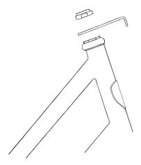
Unscrew the large, flat, nut pictured above. Remove the thin spacer (if present) and place your L-shaped bracket that comes with the basket as pictured. Fasten with the previously removed large, flat, nut.
