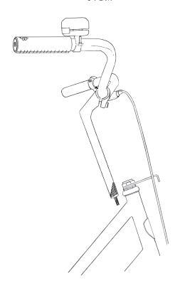
Put the stem in the frame and adjust to the desired height, but never higher than the maximum height indicated on the stem.
