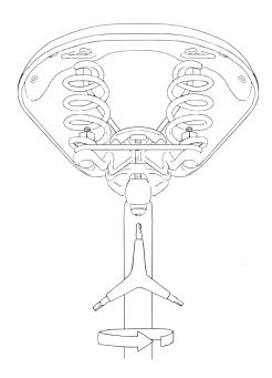
Fit the saddle to the seat post, first loosen the screw on the bottom enabling you to turn the top plate 45°. Assemble the saddle front to back and turn the top plate in place. When the seat is in position tighten the screw so the saddle rails are pressed into the grooves between the plates.
