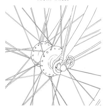
Tighten the wheel nuts clockwise - for both sides - with a 15mm spanner. Attach the fender's stays in the front fork as illustrated using the screws included. Tighten the screws clockwise - for both sides - with a 4mm allen key.
