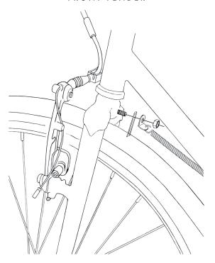
Unscrew the front wheel's two wheel nuts and place the front forks over the wheel's axle (the washers must be on the outside of the front fork). Attach the front fender as illustrated.
