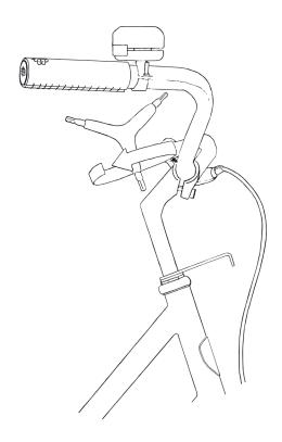
Fasten the stem by tightening the screw on the top with a 6mm allen key.
