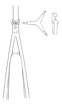
Put the seat post in the frame and adjust to the desired height. Fix the seatpost by tightening the right screw (rear view) clockwise with a 5mm allen key. The screw on the opposite side has a groove that locks the screw onto the frame.
