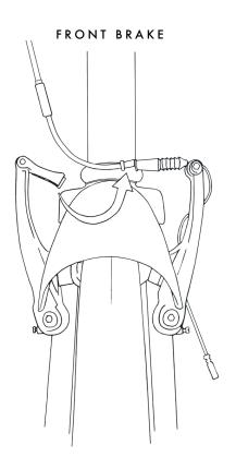
Close the brake by pinching the brake arches together and squeeze the end cap into the cable hook unit. Squeeze the brake lever a few times to ensure everything is in the right position and working properly.
