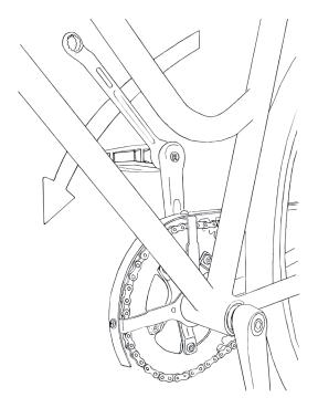
Assemble the pedals on the crank. The pedals are marked with R (right) or L (left). The right pedal is tightened clockwise, and the left counterclockwise, using a 15mm wrench.
